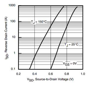
Fig 9. Typical Source-Drain Diode Forward Voltage
