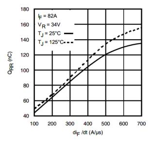
Fig 20. Typical Stored Charge vs. dif/dt
