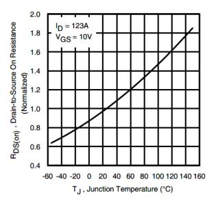
Fig 6. Normalized On-Resistance vs. Temperature
