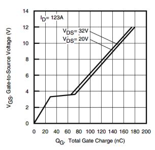
Fig 8. Typical Gate Charge vs. Gate-to-Source Voltage
