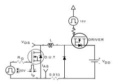
Fig 23a. Unclamped Inductive Test Circuit
