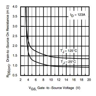
Fig 1. Typical On-Resistance vs. Gate Voltage
