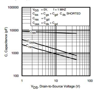
Fig 7. Typical Capacitance vs. Drain-to-Source Voltage
