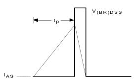
Fig 23b. Unclamped Inductive Waveforms
