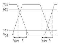
Fig 24b. Switching Time Waveforms
