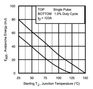
Fig 16. Maximum Avalanche Energy vs. Temperature
