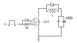
Fig 25a. Gate Charge Test Circuit
