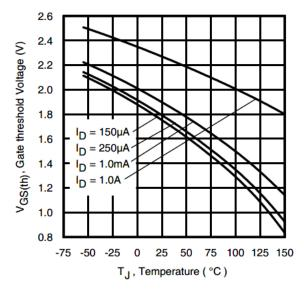
Fig 17. Threshold Voltage vs. Temperature
