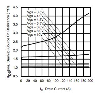
Fig 13. Typical On-Resistance vs. Drain Current
