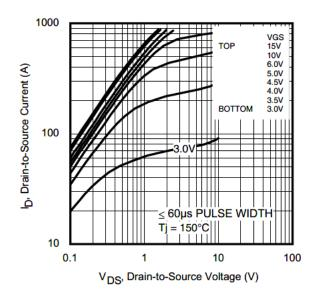
Fig 4. Typical Output Characteristics
