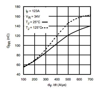
Fig 21. Typical Stored Charge vs. dif/dt
