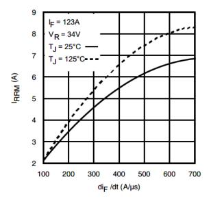
Fig 19. Typical Recovery Current vs. dif/dt
