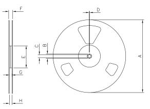
NOTE: Controlling dimensions in mm Std reel quantity is 4800 parts. Ordered as IRL7486MTRPBF
