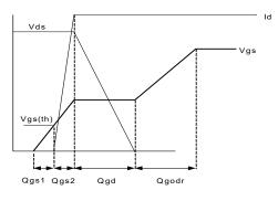
Fig 25b. Gate Charge Waveform
