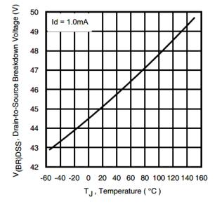
Fig 11. Drain-to-Source Breakdown Voltage
