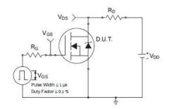
Fig 24a. Switching Time Test Circuit
