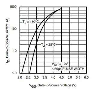
Fig 5. Typical Transfer Characteristics
